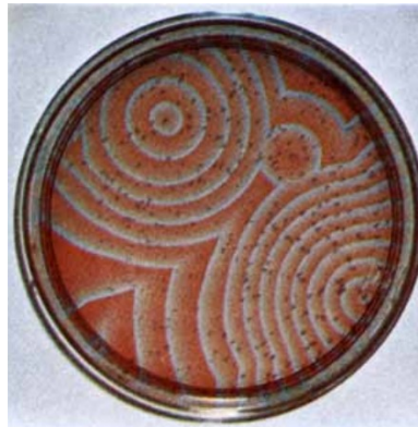
FIG. 1: Target patterns in BZ reaction, from [2]. Periodic "trigger" waves propagate from imperfections in the solution. The imperfections can under some circumstances be removed, leaving the reagents in a steady state.
